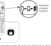
4. Place the handset onto the base (or charger) as shown. An animated battery icon will display after a few minutes to show that the handset battery is successfully being charged. For optimum performance, please allow the battery to charge for 16 hours
