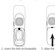
. Align the cover against the battery compartment and slide it upwards until it clicks
