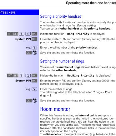
When this feature is active, an internal call is set up to a specified handset as soon as the noise in the monitored room reaches the pre-defined level. You can hear the noise in the room when you pick up the call. The room monitor remains active even after the handset is replaced. Calls to the room mon-
